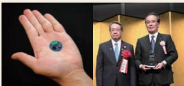
**Amcenna** – a miniature and low-profile 2.4GHz frequency antenna that can be mounted on metallic objects without degrading antenna characteristics
