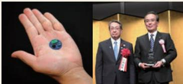
Amcenna – a miniature and low-profile 2.4GHz frequency antenna that can be mounted on metallic objects without degrading antenna characteristics
